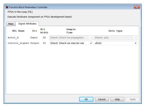
Example of FIL Block Mask Signal Attributes Tab (Generated From HDL Code)
